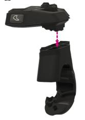
Screw remote back onto its holder (0.5Nm) using the new screws (M3x10).
