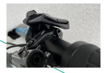
With some brakes, the clamp of the brakes can collide with the underside of the Remote Basic, if the brake is to be applied more steeply. To avoid this, we have created a spacer that increases the distance and allows space for individual brake adjustment:
