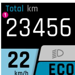
1. Odometer (total number of kilometres that the e-bike has covered. This value cannot be reset.)
